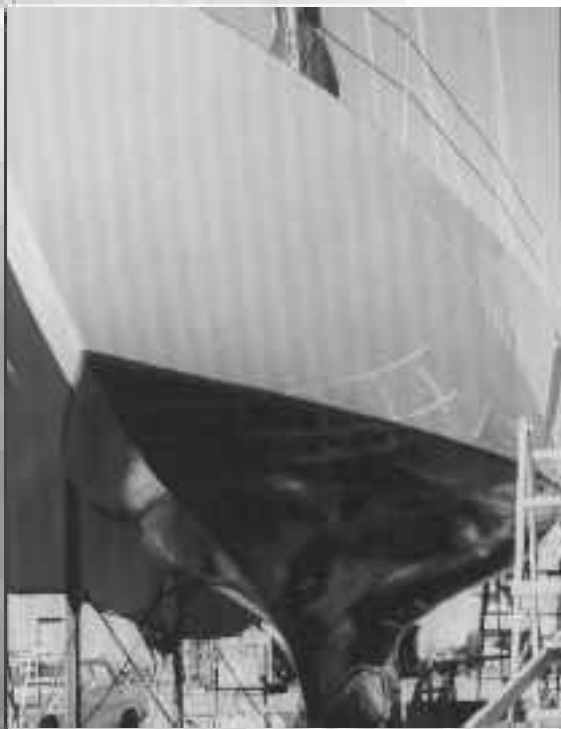
Composite materials are used in the hull and deck
